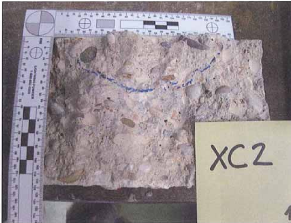
Picture 2: CEM III-A: Coated, subjected to one pressure cycle (20 bar resp. 290.1 psi over 72 h)
