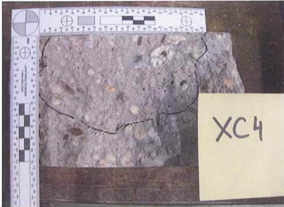
Picture 4: CEM II-A/V: Uncoated and subjected to two pressure cycles (20 bar resp. 290.1 psi over 72 h)
