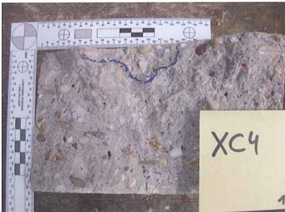
Picture 5: CEM II-A/V: Coated and subjected to one pressure cycle (20 bar resp. 290.1 psi over 72 h)
