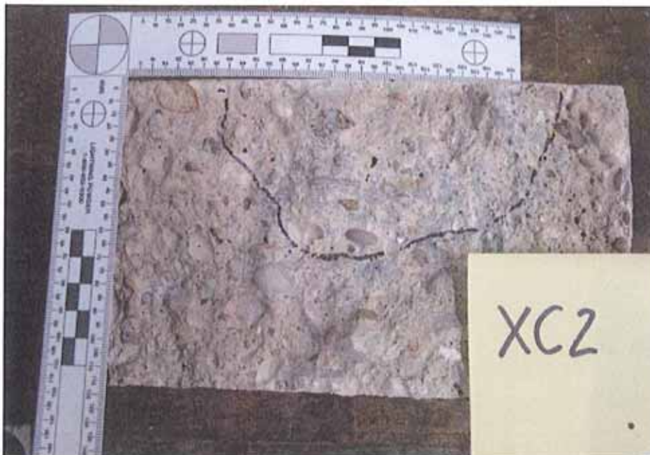
Picture 1: CEM III-A: Uncoated and subjected to two pressure cycles (20 bar resp. 290.1 psi over 72 h)
